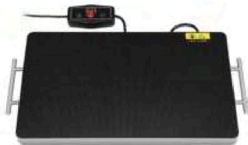
Dish Warmer Table Top Size: 560 × 305 × 45 mm Power: 350w Temp. Range: 0 - 80 °c
